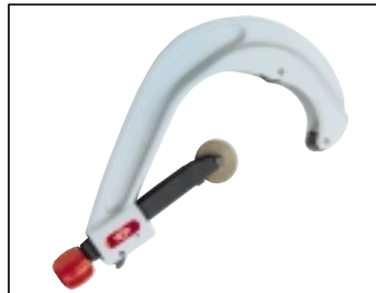
WIDOS pipe cutting equipment size 1, 6-63 mm Art.-No. W550100 0,7 kg size 2, 50-116 mm Art.-No. W550110 1,5 kg size 3, 110-168 mm Art.-No. W550120 1,7 kg Replacement cutter wheel size 1 Art.-No. W550101 0,05 kg Replacement cutter wheel size 2 + 3 Art.-No. W550111 0,05 kg
