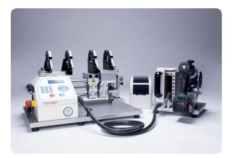
The **SP63M Mobile** is an automatic welding machine for heating element infrared welding of PE, PP, PVDF and ECTFE pipes and fittings from OD 20 to OD 63 mm in the workshop or in the field. It's portability allows it to perform welds in difficult to reach areas. It has two large aluminum pipe clamps which accept reducers for different pipe sizes, as well as two narrow fitting clamps for fittings with short legs.
